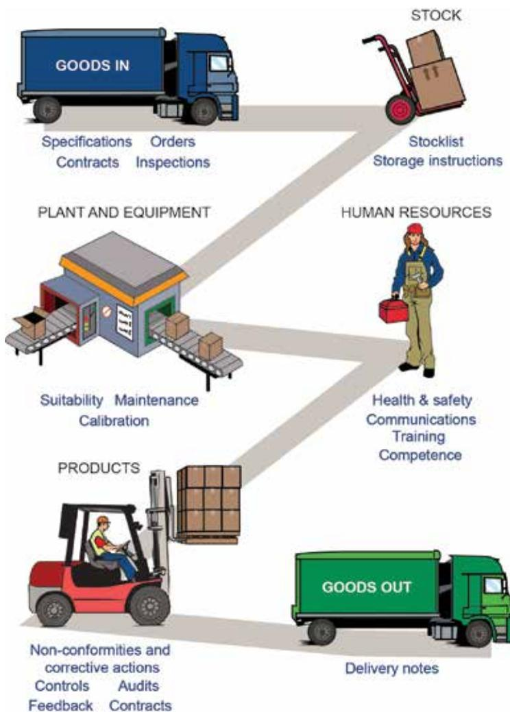
**Figure 1:** FPC documents describing the quality of production in the factory, from goods inwards to good outwards
